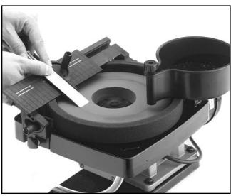
Figure 6. Typical wet wheel grinding operation.
